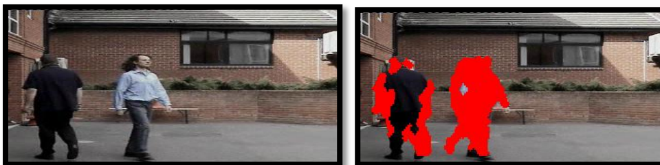
Fig.2. Temporal differencing sample. (a) A sample scene with two moving objects. (b) Temporal differencing fails to detect all moving pixels of the object on the left hand side since it is uniform colored. The detected moving regions are marked with red pixels. Processing
