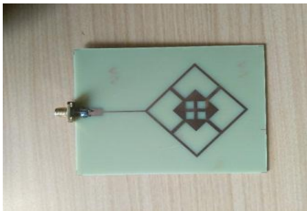
Fig 2 Front and back view of Rhombus shaped Microstrip antenna without capacitor
