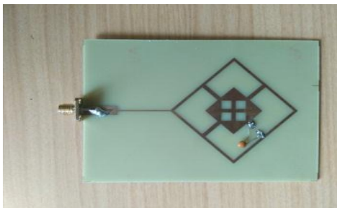
Fig 3 Front and back view of Rhombus shaped Reconfigurable Microstrip antenna with capacitor
