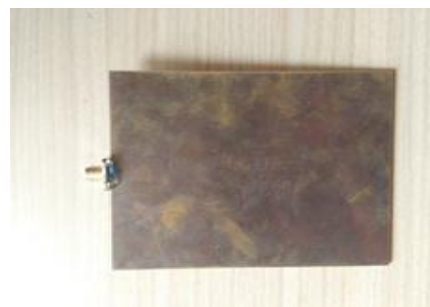
Fig 3 Front and back view of Rhombus shaped Reconfigurable Microstrip antenna with capacitor
