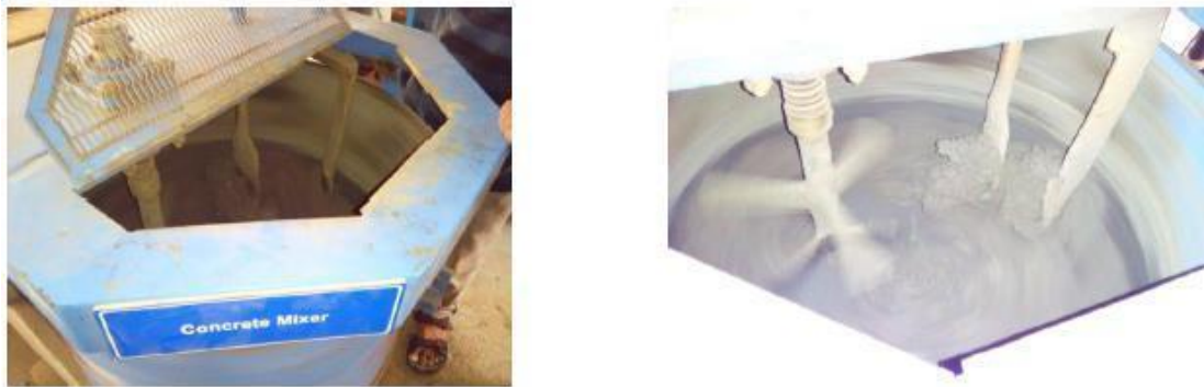
Fig2. Preparation of mix in a concrete mixer
