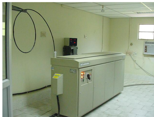
Figure.1. Solid state Nd:YAG Laser source at WRI used for experimental work (WRI 2008).
