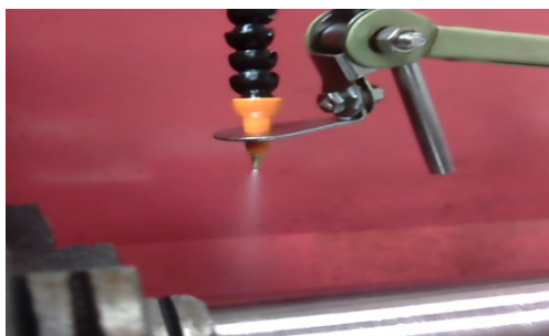
Fig.2.c: MQL Nozzle supplying mist
