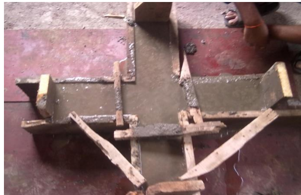
Fig. 10 Casting specimen with mold.
