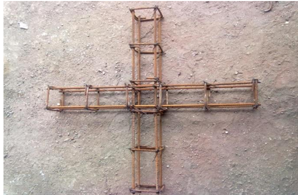
Fig. 9 Reinforcement details for test specimen.
