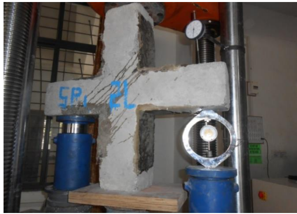
Fig. 5 Test arrangement for Rehabilitated specimen.
