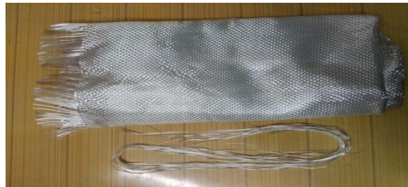
Fig 2.2.1 - Fibre glasses are in different physical forms like microspheres, chopped or woven fiber.
