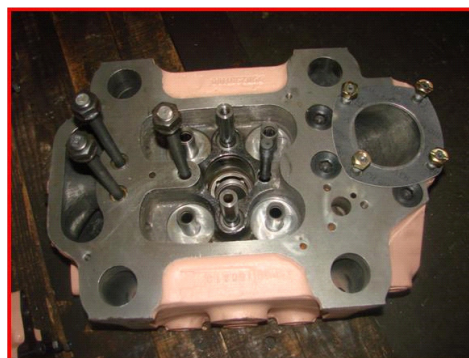
Fig.3 Valve Guide fitted into Cylinder Head
