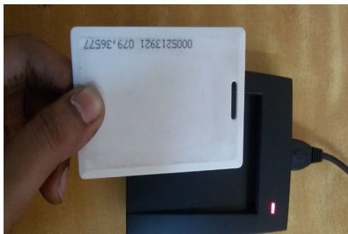
Fig (3): RFID Tag being scanned by the RFID Reader
