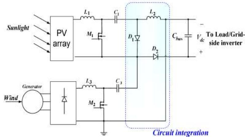
Figure 4: Proposed Bi-input rectifier stage topology.
