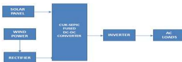
Figure 3: Block Diagram for Cuk SEPIC fused Topology.
