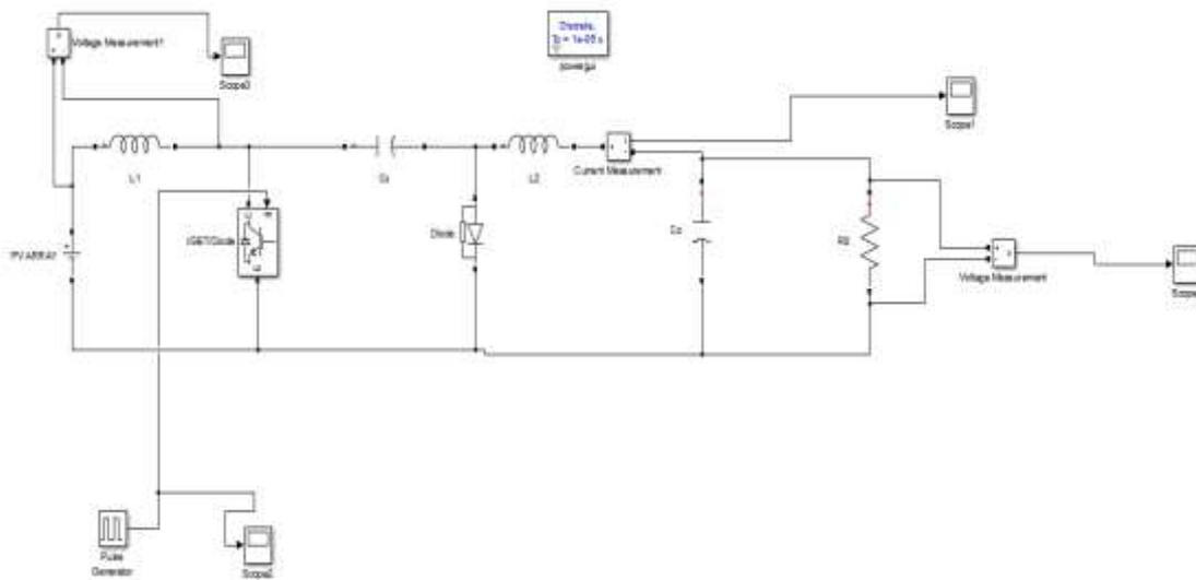
Figure 10: Simulink Model of Cuk converter.
