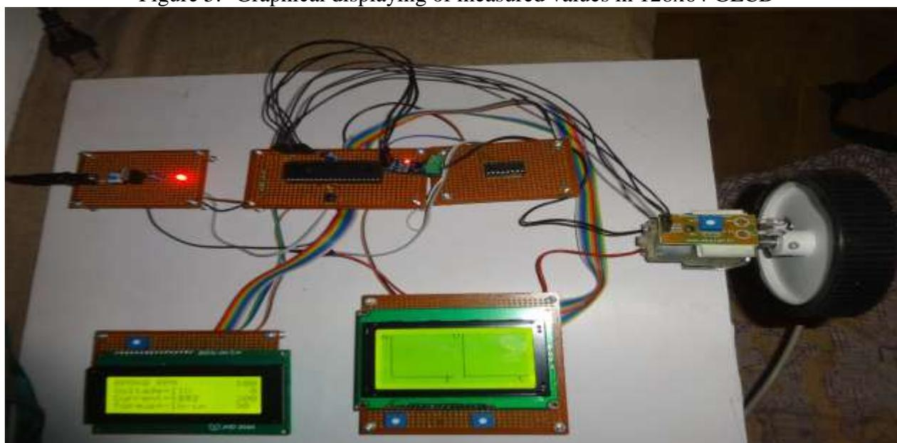
Figure6:-Project Model of measurement, protection, speed control and graphical observation of dc motor
