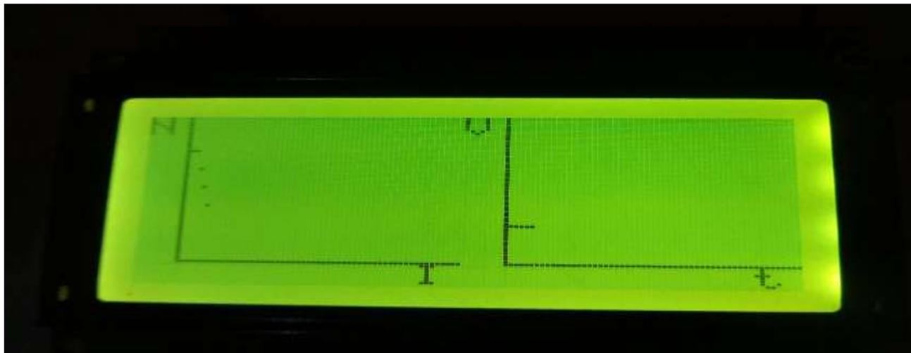
Figure 5:- Graphical displaying of measured values in 128x64 GLCD
