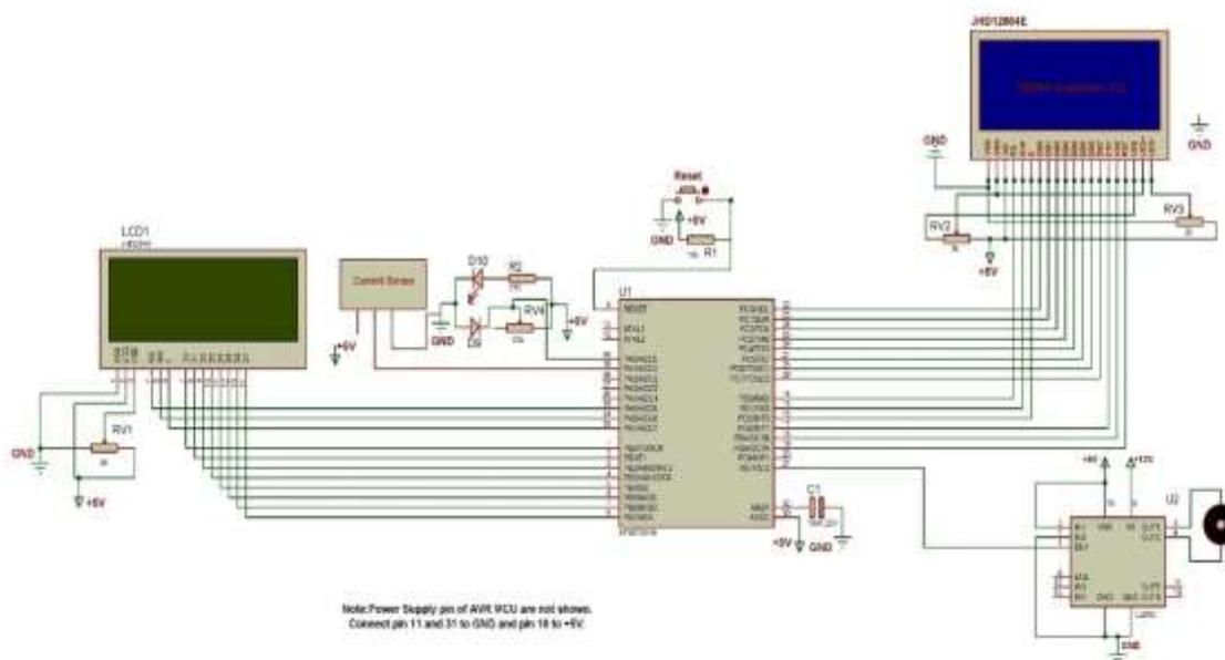
Figure 2:- Circuit diagram of measurement, protection, speed control and graphical observation of dc motor
