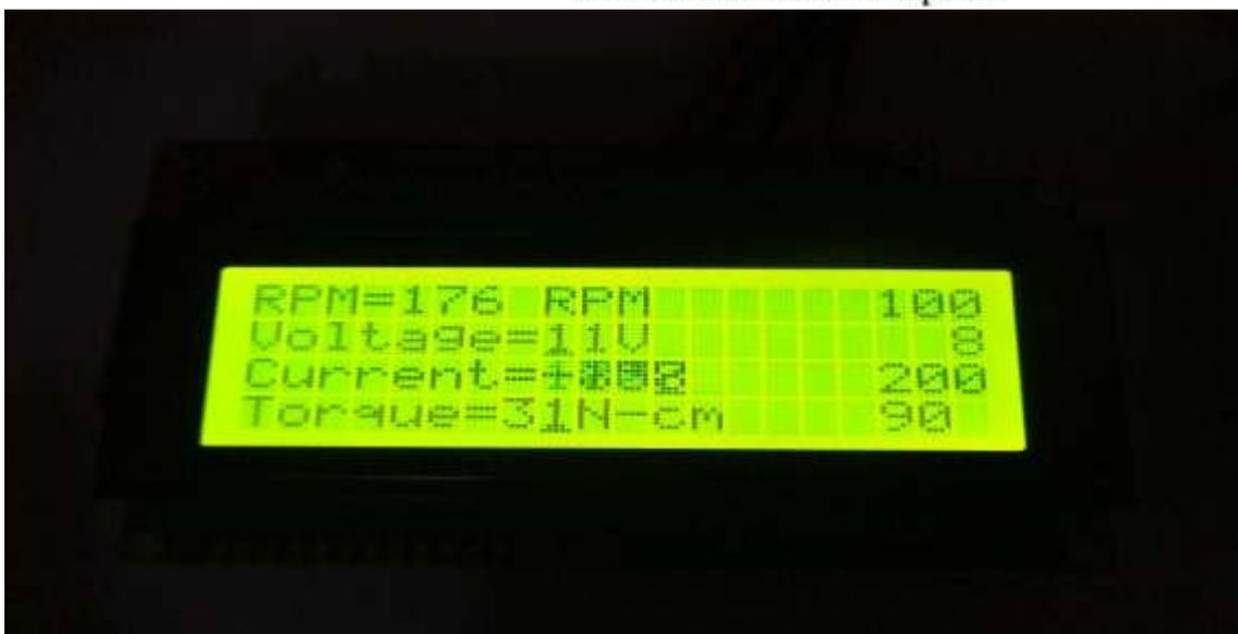
Figure 3:- 16X4 LCD displaying parameters value and limit values
