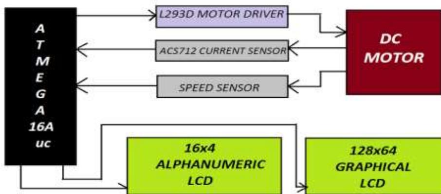
Figure 1:- Block diagram of measurement, protection, speed control and graphical observation of dc motor
