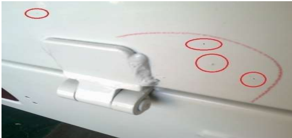
Fig.2. Stucked spatters on tail gate panel of a truck cargo.
