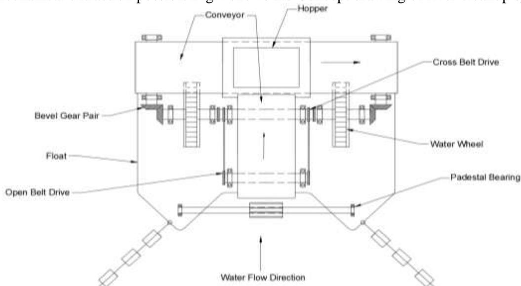
Fig. 4. Concept drawing of river cleanup system.
