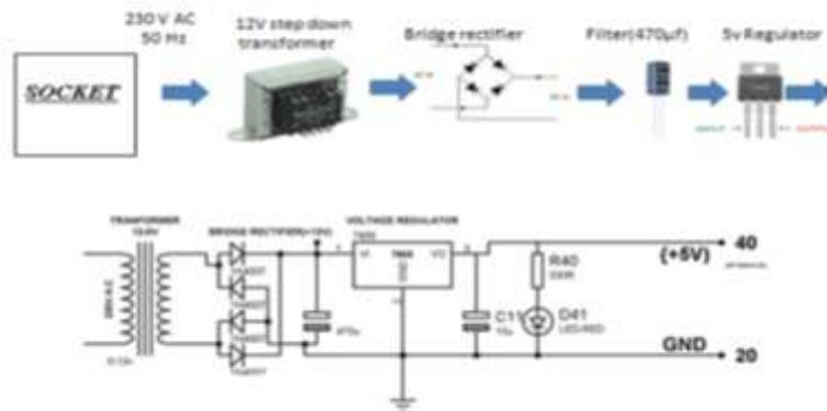
Fig. 2. Circuit Diagram of Power Supply Block of Four Quadrant DC Motor Control
