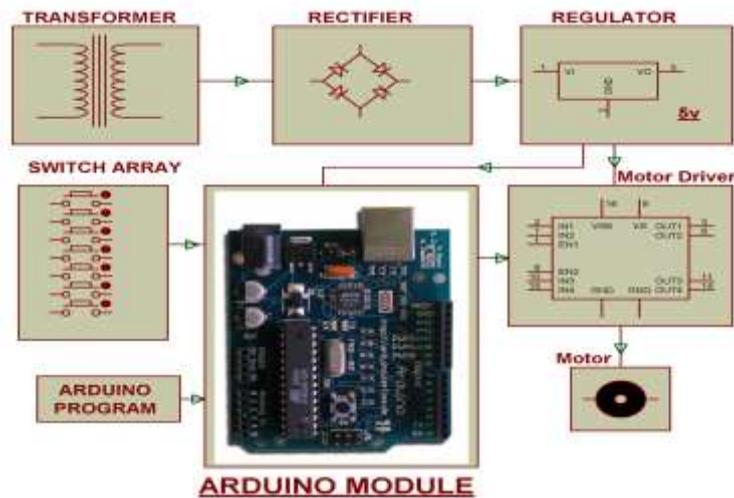
Fig. 1. Block Diagram of Four Quadrant DC Motor Speed Control By Using Arduino
