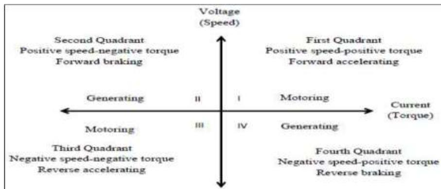
Fig. 4. Four Quadrant Operation of a DC Motor
