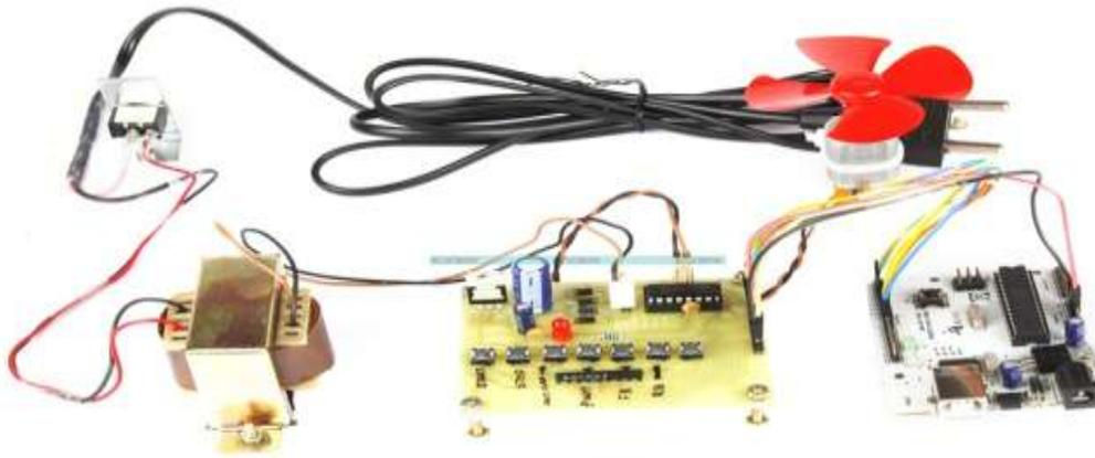
Fig. 5. Practical Implementation of Speed Control Dc Motor
