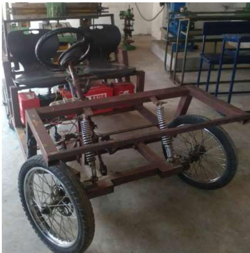
**Figure.15 Free powered electric vehicle working model**
