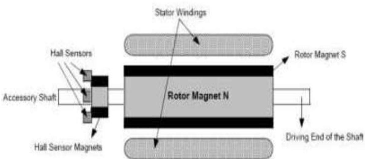
**Figure.3 Motor Mechanical Structure**
