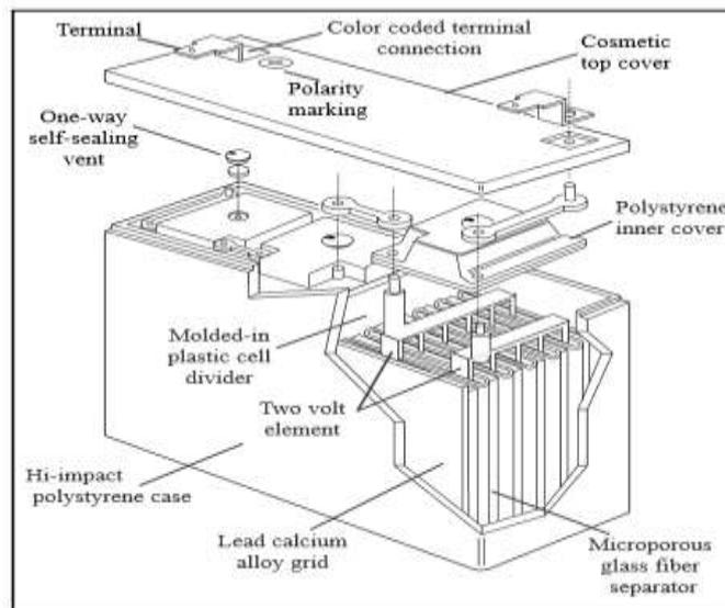
**Figure.5 Construction of battery**
