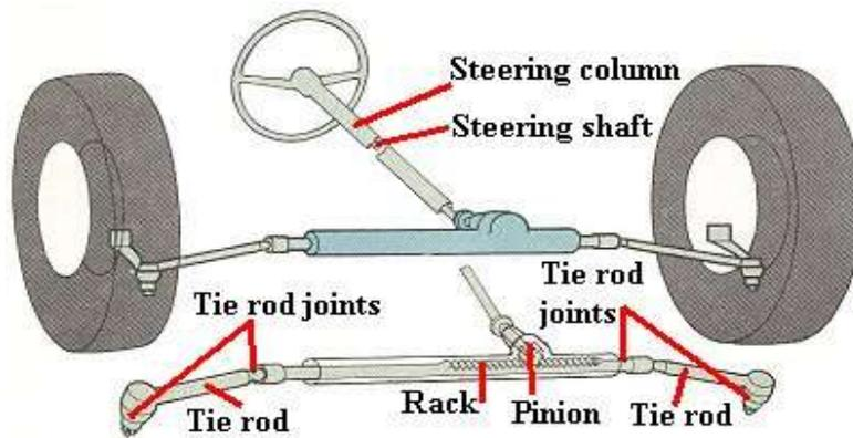
**Figure.10 Front Wheels, Basic components of steering system Supporting channel for steering mechanism and front wheel connection**
