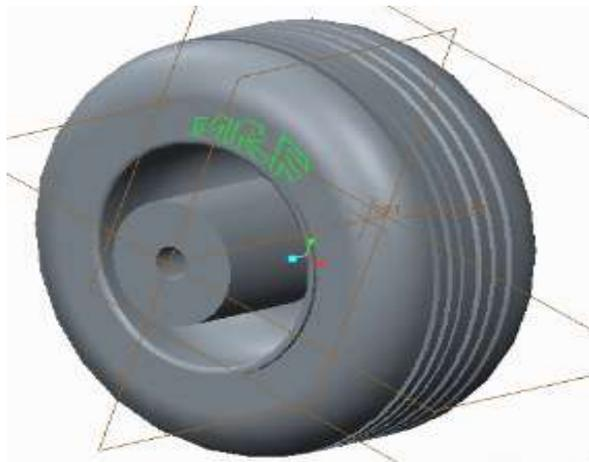
**Figure.4 Hub Motor Wheel**
