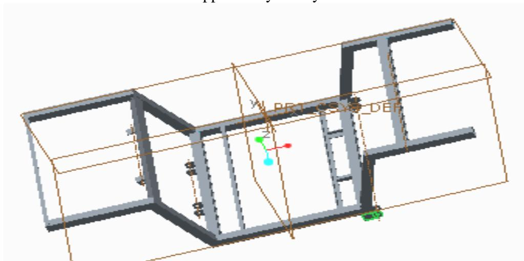
**Figure.8 Chassis of electrical vehicle**
