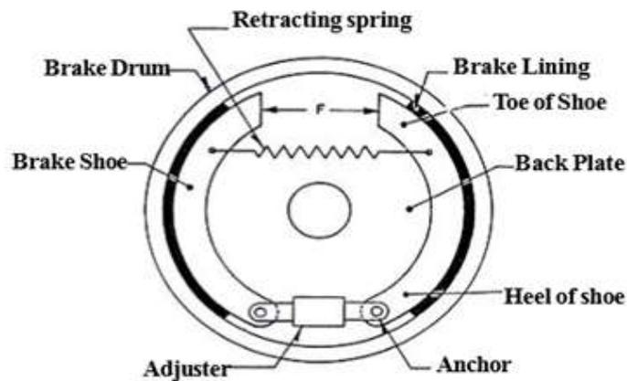
**Figure.13 Drum brake**
