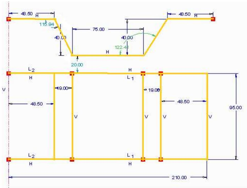
**Figure.9 Line Diagram Chassis Dimensions**
