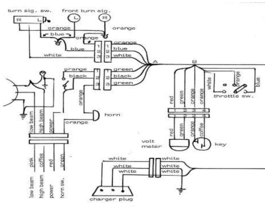
**Figure .7 Electrical Wiring of an Electrical Vehicle**
