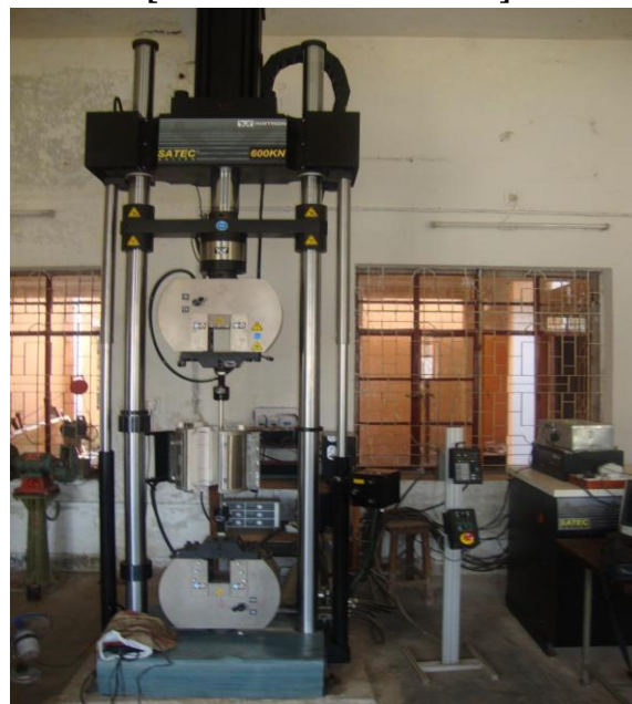
Fig 2: Hot Tensile Testing Set-Up-INSTRON static [7]
