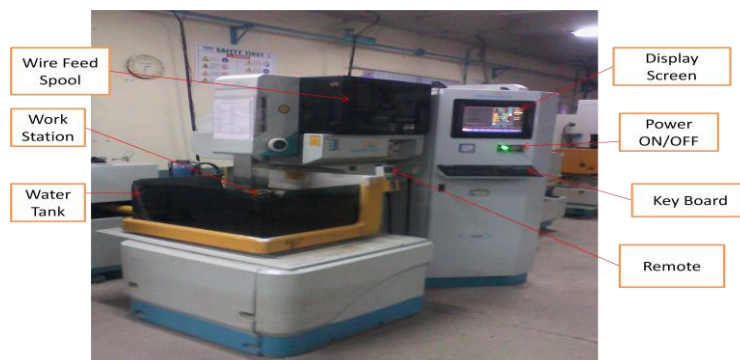
Figure 3: Pictorial View of WEDM Experimental Setup.
