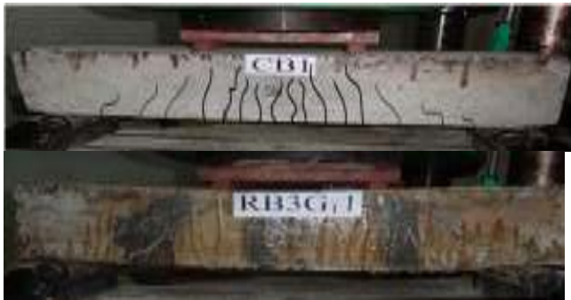
Fig. 5 – Failure patterns for beams
